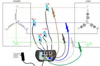
Connection to 3-phase 4-wire system
