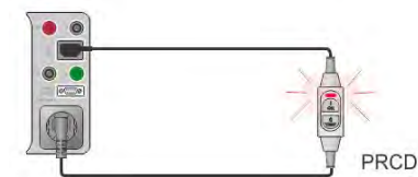
Active polarity test
