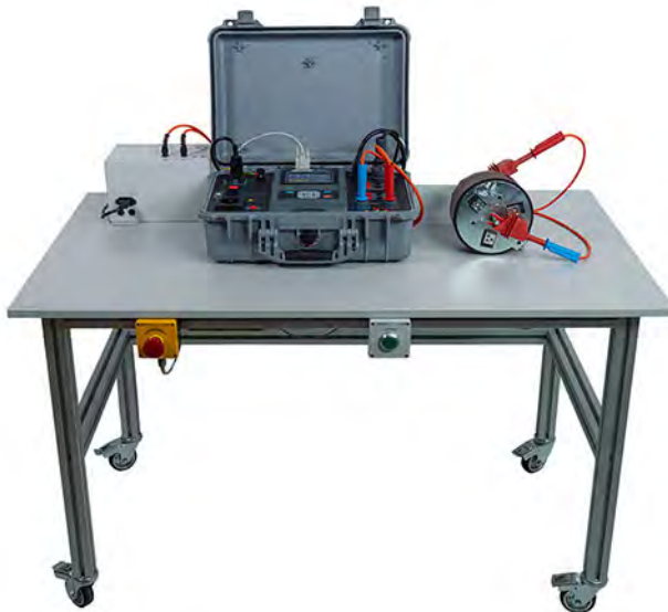
S 2115 safety system with current limitation I_{test} < 3\text{mA}
