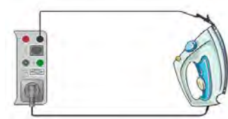
Substitute leakage test for Class I device
