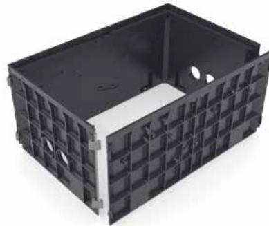
**STEP 5** – If required, build a second chamber section and stack it on top of the first section. Knock corners into place until they are tightly matched.
